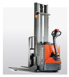
An electric stacker, also known as a walkie stacker, is a power-propelled device for lifting and loading pallets. Primarily a stacker is used to lift, move and stack pallets on a shelf at a high level. This type of device is mostly found in warehouses.
