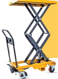
Mobile hydraulic scissor lifts are typically small, lightweight units that can push goods or heavy objects around a factory or workshop.
