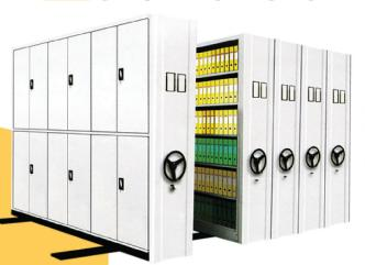
Mobile compactor storage systems are mounted onto light or heavy-duty base units which can be moved in a parallel direction to each other. The system runs on two rails provided for the whole length of the unit. The system requires only one aisle to provide access to all items in stock. This type of system increases the storage capacity and reduces the floor space occupancy.
